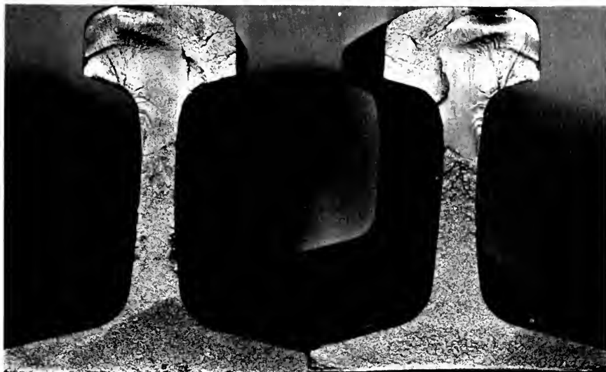
Fig. 5—Fractured faces of electric flash butt welded rail joint, specimen 225C, that failed after being subjected to 1,438,400 cycles of repeated loading in the 12-in stroke rolling-load machine under a 57,500-lb wheel load. This fatigue failure originated in the fillet between the head and web and is the result of a shear drag.
